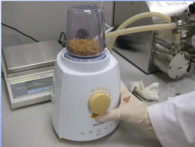
Grinding dried wheat grains
