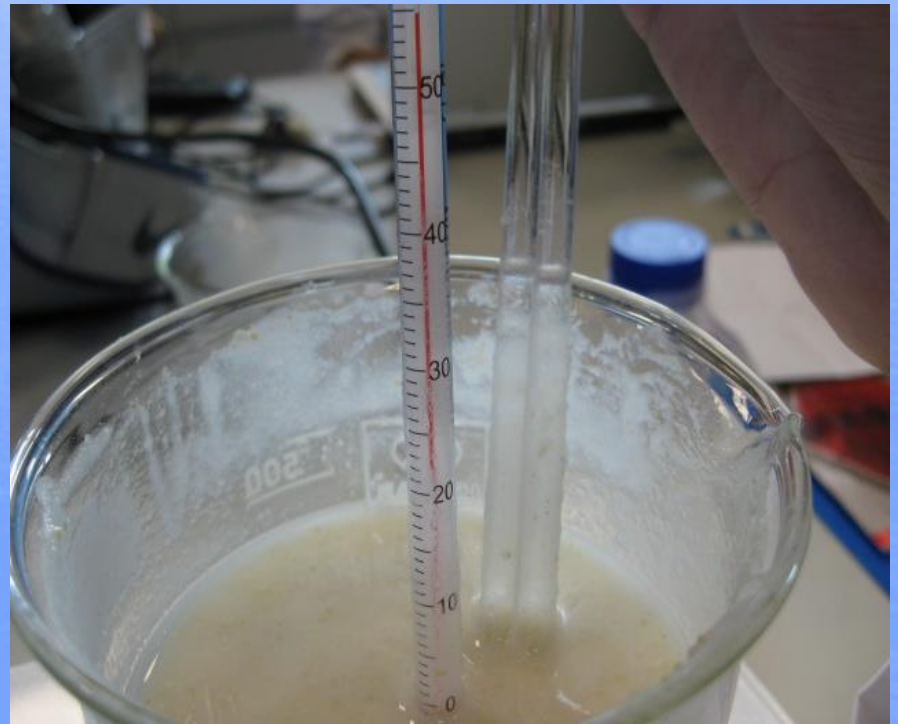
Saccharification [starch to sugar]
